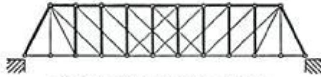
(e) THROUGH WHIPPLE TRUSS
